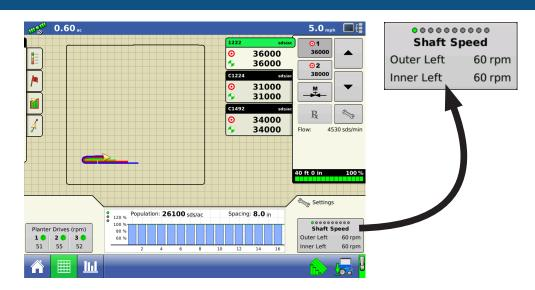
Auxiliary sensors in bottom right. Touch box to cycle through other sensors.
